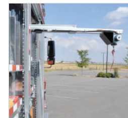
SIDE MOUNTED WINCH When confined by height, a side mounted winch is a good solution for removing heavy and awkward equipment.
