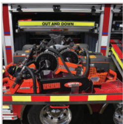
SINGLE DIRECTION SLIDE Extends up to 100% and features a 1,000-lb. capacity.
