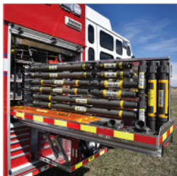
DUAL-DIRECTION SLIDE Features 70% extension and up to 1,000 lbs. of capacity.
