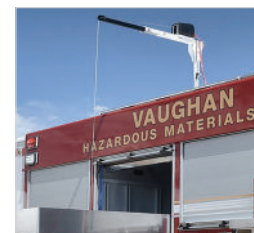
OVER-HEAD WINCH For heavy equipment, when there are no height restrictions.
