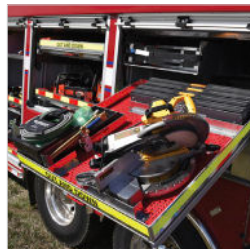
SLIDEOUT TILT-DOWN Provides 30-degree access for high storage areas.
