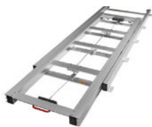
83 SERIES Heavy-duty cargo slides feature up to 1,000 lbs. of capacity and 70% extension and are available in 40-96" depth.
